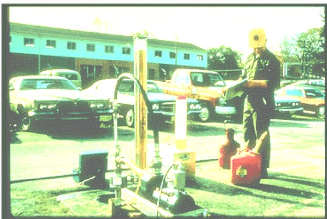
Tank tightness testing is a good way to determine if an existing heating oil tank is leaking. Remember, most heating oil tanks last only 10 to 15 years before replacement is needed.
